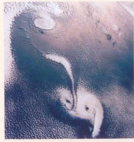
This space shuttle photograph, taken near the island of Guadeloupe in the Caribbean Sea, shows swirling cloud formations in an atmospheric phenomenon known as a Von Karman vortex street. The long line of eddies that rotate alternately clockwise and counterclockwise is caused by obstacles, such as islands, disturbing the airflow as it passes over them. Von Karman vortex streets are often seen in satellite images of clouds.
